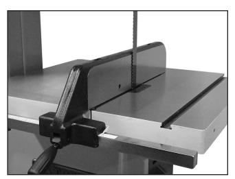
Figure 11. Fence flush with blade.
